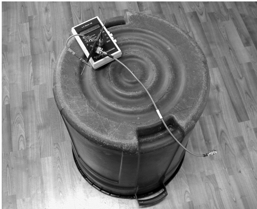
Figure 3 — Shunt capacitance measurement of the center fitting.
