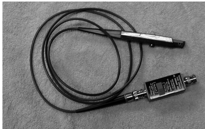
Figure 34 — Scope probe used for current pickup.
